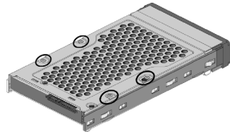
Figure 2-4-2. Installing 3.5-inch SAS/SATA Drive
