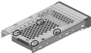
Figure 2-4-1. Installing 2.5-inch SAS/SATA Drive
