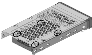
Figure 2-4-1. Installing 2.5-inch SAS/SATA Drive
